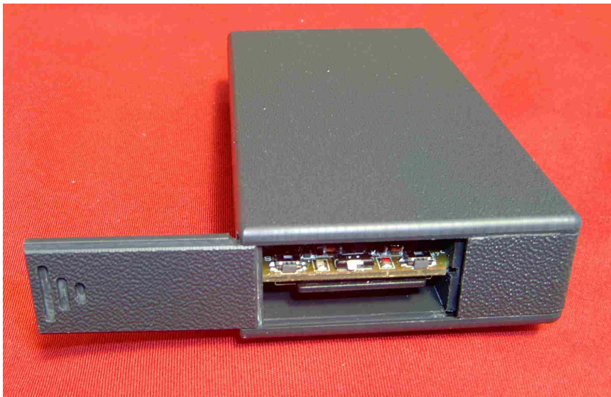
Figure 2 Rear View with Slide Open showing Second On / Off slider switch with two other special mode control buttons on either side.
